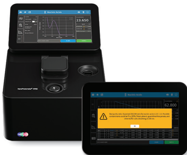
Figure 1: NanoPhotometer® NP80 and a warning screen “Bad purity ratio. Expected 260/230 ratio for nucleic acids is 2.0 – 2.2. Possible contaminants could be Tris, EDTA, Trizol, phenol, guanidine thiocyanate, and other buffer salts absorbing at 230 nm.”
